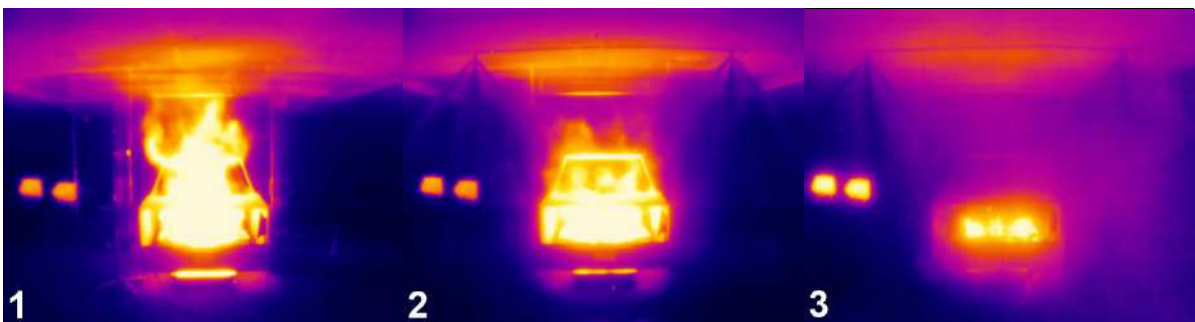
Thermal images of vehicle fire tests with water mist activation
