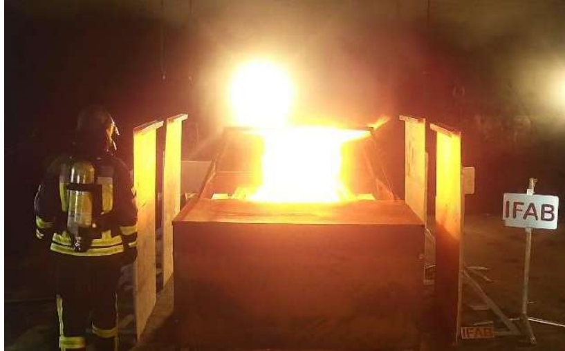
Water mist activation in SUVEREN fire test with electric vehicle
