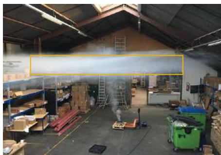
(a) Stratification of a TF2 test during a summer day in a warehouse facility
