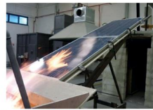
UL 1703 spread of flame test orientation.
